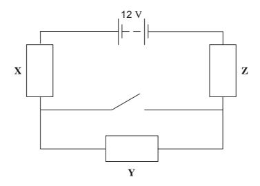
With the switch open, as shown, the current in resistor Y is 20 mA. When the switch is closed, what is the current in resistor X, and what is the potential difference (voltage) across resistor Z?
